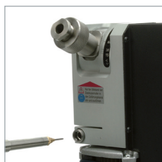
Precise adjustment of the electrode's stick-out.
